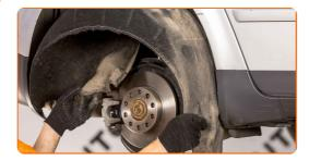
Unscrew the upper fastener of the shock absorber. Use HEX No.H6. Use a ratchet wrench.
