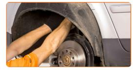
Install and tighten the wheel arch cover fasteners. Use Torx T25. Use a ratchet wrench.
