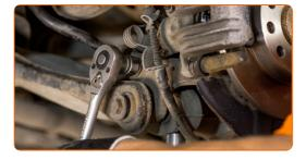
Tighten the lower fastener of the shock absorber. Use a drive socket #21. Use a torque wrench. Tighten it to 150 Nm torque.+90°
