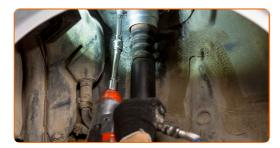
Screw in the lower fastener of the shock absorber. Use a combination spanner #21. Use a drive socket #21. Use a ratchet wrench.
