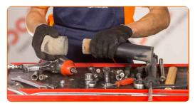
17 Remove the shock absorber dust cap and the bump stop.
