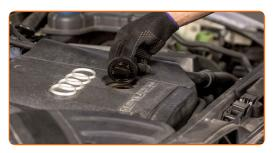
Tighten the oil filler cap.
