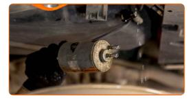
Put the old filter cartridge in the container.
