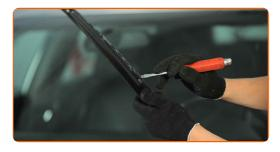
Remove the blade from the wiper arm.
