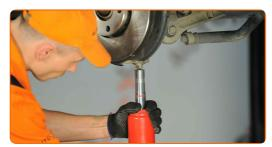
Tighten the lower fasteners connecting the shock strut to the steering knuckle. Use a combination spanner #18. Use a drive socket #18. Use a torque wrench. Tighten it to 90 Nm torque.
