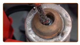
Remove the strut piston rod nut. Use a drive socket #18. Use a ratchet wrench.
