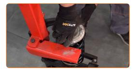
Release the coil spring.
