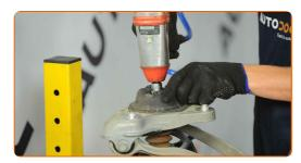
Remove the top mount, the support bearing and the upper spring cup.
