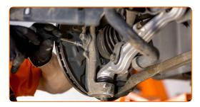
Tighten the drive shaft nut. Use HEX No.H17. Use a torque wrench. Tighten it to 115 Nm torque.+180°
