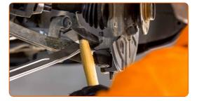
Loosen the tie rod end fastening bolt. Use a drive socket #13. Use a ratchet wrench.
