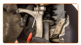
Unscrew the ABS sensor fastening from the steering knuckle. Use a drive socket #10. Use a ratchet wrench.
