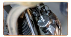
Unscrew the caliper bracket fastening. Use a drive socket #21. Use a ratchet wrench.
