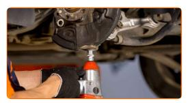
Connect the tie rod end to the steering knuckle. Use a hammer.
