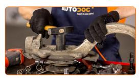
Unscrew the hub bearing fastening to the steering knuckle. Use XZN #12. Use a ratchet wrench.
