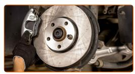
Tighten the brake caliper bracket. Use a drive socket #21. Use a torque wrench. Tighten it to 190 Nm torque.
