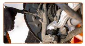
Remove the ABS sensor from the steering knuckle.
