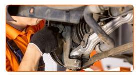
Screw in the fastener that connects the ABS sensor to the rear knuckle. Use a drive socket #10. Use a ratchet wrench.
