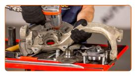
Press out the wheel hub bearing. Use a hammer.
