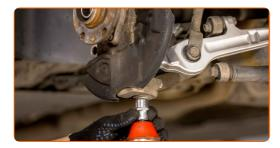
Disconnect the lower arm from the steering knuckle. Use a hammer. Use a crowbar.
