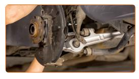
32 Screw the wheel hub axle nut.
