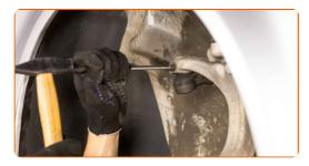
Disconnect the tie rod end from the steering knuckle. Use a flat metal-working chisel. Use a hammer.
