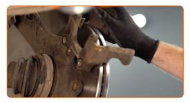
18 Remove the brake disc.
