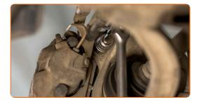
Connect the brake pad wear sensor plug.
