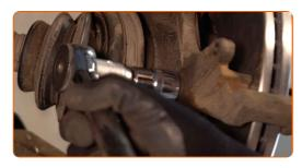
17 Remove the caliper bracket.
