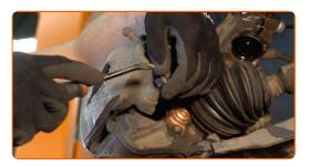
Disconnect the brake pad wear sensor plug. Use a flat screwdriver.
