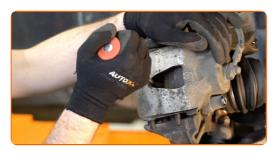
13 Remove the brake caliper.
