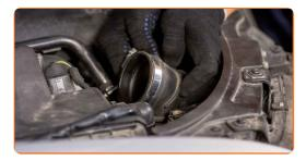
16 Install the air duct housing.
