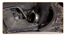
Detach the vacuum pipe. Use a flat screwdriver.
