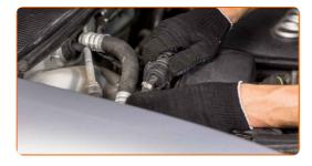
Install the air intake pipe and secure it. Use a flat screwdriver.
