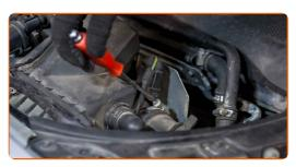
6 Remove the air intake pipe.
