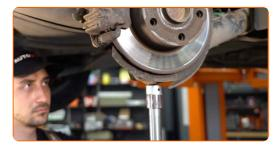
Tighten the lower fastener of the shock absorber. Use a combination spanner #16. Use a drive socket #16. Use a torque wrench. Tighten it to 50 Nm torque.+90°
