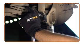
9 Remove the fastening bolt.
