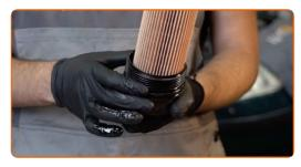
Screw the new filter into its place.
