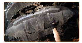
Tighten the fasteners of the oil pan lower cover. Use a drive socket #10. Use a ratchet wrench.
