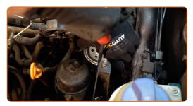
Install and tighten the cap of the fuel filter housing.
