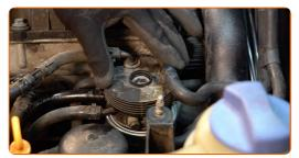
Tighten the fasteners of the fuel filter housing cover. Use HEX No.H13. Use a torque wrench. Tighten it to 25 nm torque.
