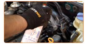
Unscrew the fasteners of the fuel filter housing cover. Use HEX No.H13. Use a ratchet wrench.
