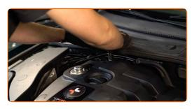
Remove the fender protection cover.
