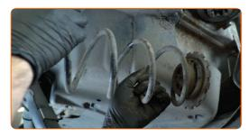
Clean the coil spring mounting seats. Use a wire brush. Use WD-40 spray.
