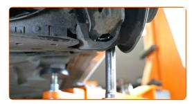
Tighten the fastener connecting the suspension arm to the rear knuckle. Use a combination spanner #18. Use a drive socket #18. Use a torque wrench. Tighten it to 85 Nm torque.
