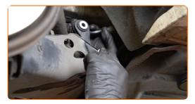
Tighten the fastener connecting the stabilizer bar with the control arm. Use a combination spanner #16. Use a drive socket #16. Use a torque wrench. Tighten it to 40 Nm torque.
