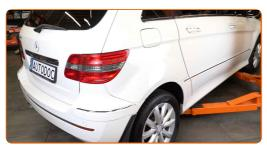
Loosen the wheel mounting bolts. Use wheel impact socket #H12.
