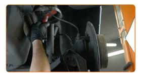
Install the coil spring together with the rubber mounts into the mounting seats.
