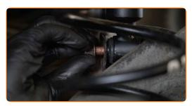
Tighten the lower fastener of the shock absorber. Use a drive socket #16. Use a torque wrench. Tighten it to 70 Nm torque.
