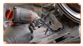
Detach the suspension arm from the rear knuckle.
