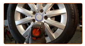
Lower the car and working in a cross order, tighten the wheel bolts. Use wheel impact socket #H12. Use a torque wrench. Tighten it to 130 Nm torque.
