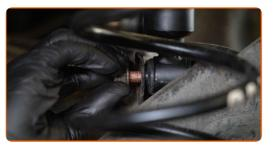
21 Screw in the lower fastener of the shock absorber. Use a combination spanner #16. Use a drive socket #16. Use a ratchet wrench.
