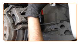
10 Remove the brake caliper.
