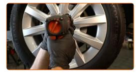
Lower the car and working in a cross order, tighten the wheel bolts. Use wheel impact socket #H12. Use a torque wrench. Tighten it to 130 Nm torque.
