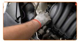
Tighten the oil filler cap.
