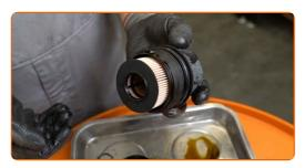
Screw the cap. Use a drive socket #27. Use a torque wrench. Tighten it to 25 Nm torque.
