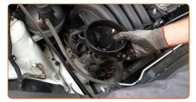
Pour oil into the engine through the filler. Required amount of oil: 5 l.
