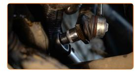
Tighten the fastener connecting the stabilizer link to the shock strut. Use a combination spanner #16. Use a drive socket #16. Use a torque wrench. Tighten it to 60 Nm torque.
