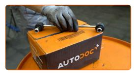
Tighten the fastener connecting the stabilizer link to the stabilizer bar. Use a combination spanner #16. Use a drive socket #16. Use a torque wrench. Tighten it to 60 Nm torque.
