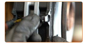
Install the brake caliper and fix it. Use a drive socket #13. Use a combination spanner #17. Use a torque wrench. Tighten it to 35 Nm torque.
