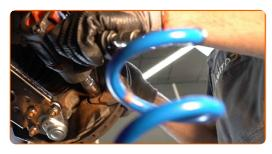
Remove the caliper bracket.
