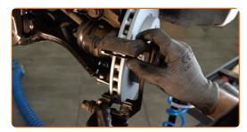
Tighten the brake caliper bracket. Use a drive socket #18. Use a torque wrench. Tighten it to 115 Nm torque.
