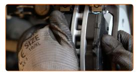
Connect the brake pad wear sensor plug.
