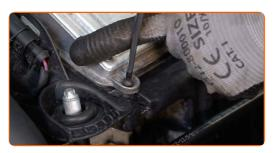
Remove the fender protection cover.
