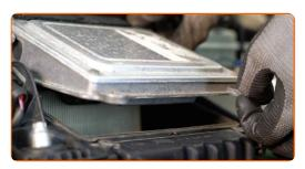
Pry up the tabs on the air filter housing. Remove the air filter housing.
