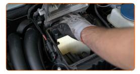
Reinstall the air filter cover. Fasten it.
