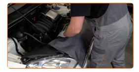
Undo the fastening screws of the air filter cover. Use Torx T20. Use a ratchet wrench.
