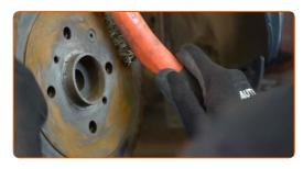
Treat the contacting surface. Use copper grease.
