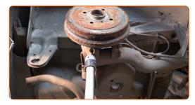
Unscrew the lower fastener of the shock absorber. Use a drive socket #17.
