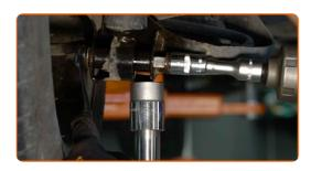
Remove the fastening bolt.
