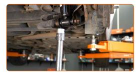
Tighten the lower fastener of the shock absorber. Use a combination spanner #17. Use a drive socket #17. Use a torque wrench. Tighten it to 75 Nm torque.
