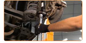
Clean the shock absorber fasteners. Use a wire brush. Use WD-40 spray.
