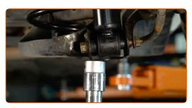
Tighten the lower fastener of the shock absorber. Use a combination spanner #17. Use a drive socket #17. Use a torque wrench. Tighten it to 75 Nm torque.
