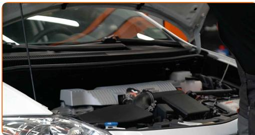
2 Use a fender protection cover to prevent damaging paintwork and plastic parts of the car.
