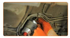
Screw the fastener attaching the fuel supply line to the fuel filter housing. Use a combination spanner #17. Use a combination spanner #22.
