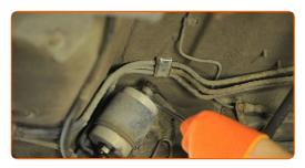
Disconnect the pipe from the fuel filter.
