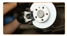
Tighten the brake caliper bracket. Use a combination spanner #15. Use a drive socket #13. Use a torque wrench. Tighten it to 35 Nm torque.
