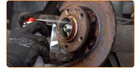
Remove the hub and the bearing together, since they are a sealed unit. Use 3-Arm Gear Puller.
