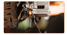
Remove the brake caliper.
