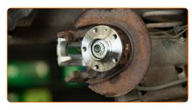
Tighten the hub. Important! Be sure to use new fasteners. Use drive 12-point socket #32. Use a torque wrench. Tighten it to 70 Nm torque.+45°
