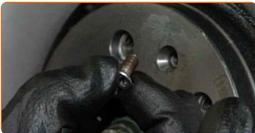
**16** Remove the brake disc.
