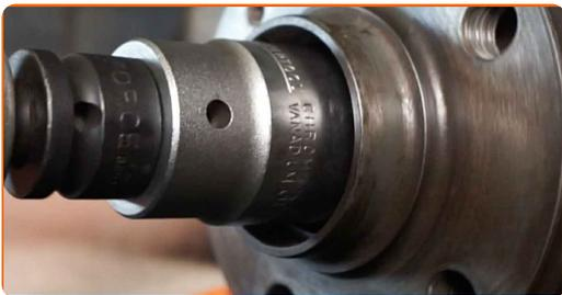
**67** Treat the ABS sensor connector. Use dielectric grease.
