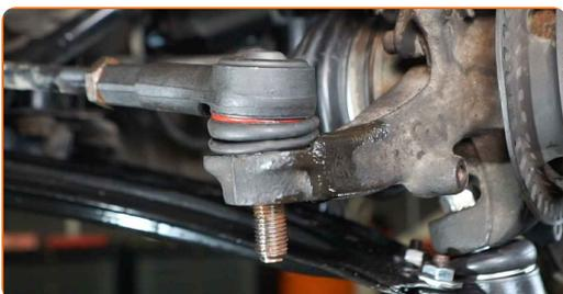
**70** Screw on the fastening nut that connects the tie rod end to the steering knuckle. Use a drive socket #19. Use a ratchet wrench.
