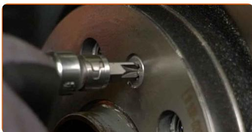
**15** Remove the fastening bolt.
