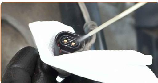
**68** Attach the ABS sensor connector.
