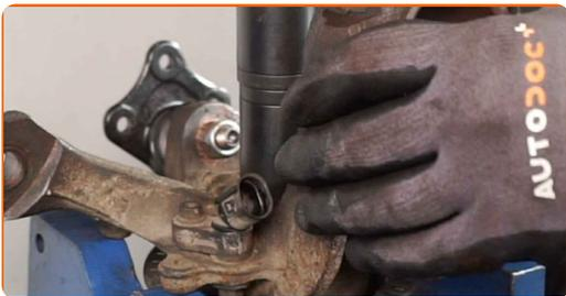
**40** Clean the wheel hub bearing retaining ring. Use a wire brush. Use WD-40 spray.
