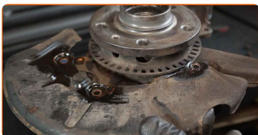
**39** Remove the wheel hub from the steering knuckle. Use a bush and bearing driver set.
