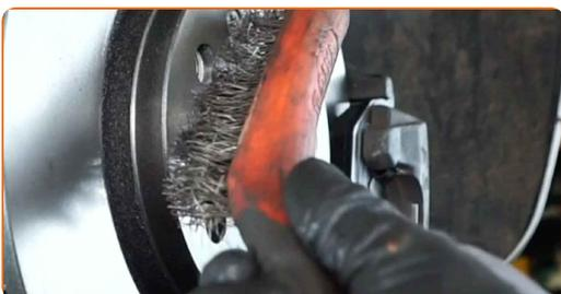
**87** Treat the surface where the brake disc contacts the wheel rim. Use ceramic grease.
