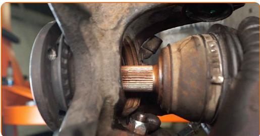
**58** Attach the ball joint to the control arm.
