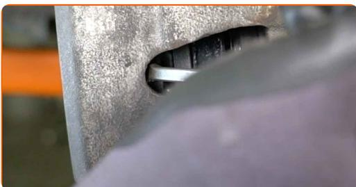
**10** Remove the caps from the brake caliper guide pin boots. Use a crowbar.
