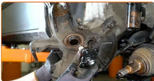
**35** Clean the fasteners of the brake disc cover. Use a wire brush. Use WD-40 spray.
