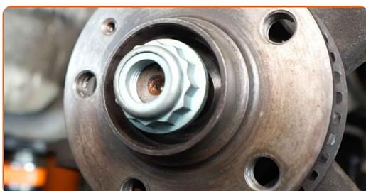
**66** Screw in the fastener of the CV axle. Use a drive socket #30. Use a ratchet wrench.
