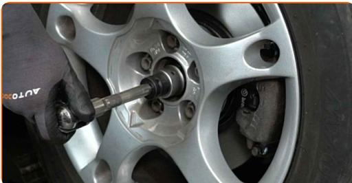
**5** Loosen the wheel bolts. Use wheel impact socket #17. Use a tap wrench.
