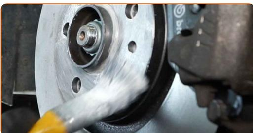
**88** Clean the brake disk surface. Use a brake cleaner.
