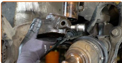
**34** Remove the steering knuckle together with the wheel hub.
