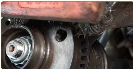
**72** Treat the contacting surface. Use ceramic grease.
