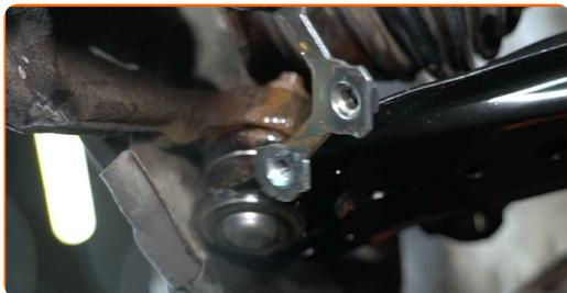
**30** Detach the driveshaft from the steering knuckle.
