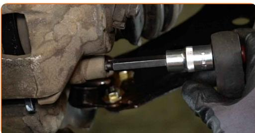
**12** Remove the brake caliper.
