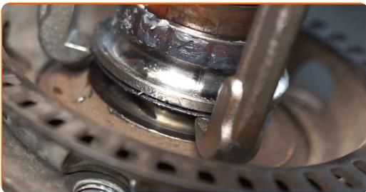
**47** Clean the wheel hub mounting seat. Use a wire brush. Use WD-40 spray.
