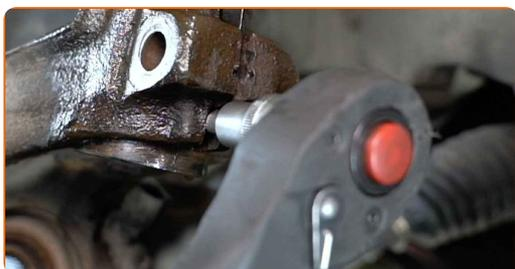
**33** Disconnect the steering knuckle from the suspension strut.
