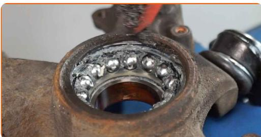
**41** Remove the wheel hub bearing retaining ring. Use circlip pliers.
