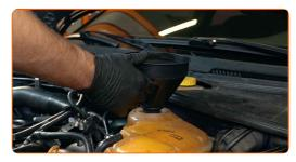
Pour coolant in the coolant reservoir.
