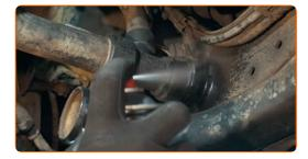
Disconnect the coolant pipe retaining clip.
