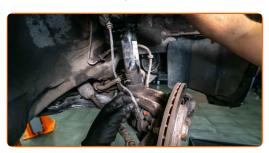
Unscrew the fastener connecting the drive shaft to the wheel hub. Use 1-3/16" drive 12-point socket.
