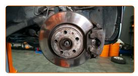
Clean the fasteners connecting the shock strut to the steering knuckle. Clean the fasteners connecting the ball joint to the suspension control arm. Use a wire brush. Use WD-40 spray.
