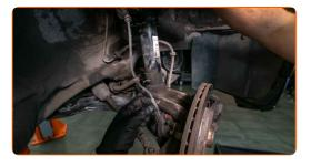
Clean the wheel rim mounting seat. Use a wire brush. Treat the contacting surface. Use copper grease. 42
