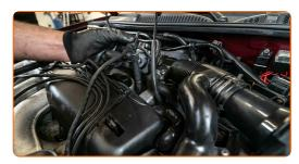
Plug in the connector on the engine intake manifold.
