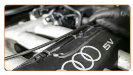
Remove the spark plug wire connectors from the spark plug wells.
