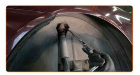
Unscrew the lower fastener of the shock absorber. Use a combination spanner #16. Use a drive socket #16.
