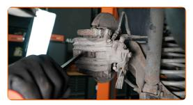
Clean the brake caliper fasteners. Use a wire brush. Use a brake cleaner.
