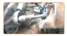
Treat the ABS sensor connector. Use dielectric grease.
