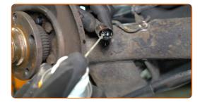
Attach the ABS sensor connector.
