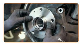
Treat the fasteners of the wheel hub bearing. Use a sealant.
