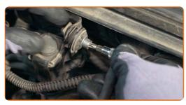
6 Unscrew the brake fluid reservoir cap.
