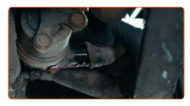
Drain the coolant from the engine.
