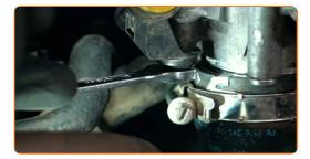
Secure the fastener of the air intake duct. Use a drive socket #7. Use a ratchet wrench.
