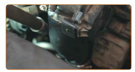
Screw in the dipstick tube fastener. Use a combination spanner #10.
