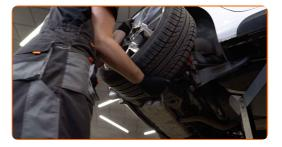
Clean the control arm fasteners. Use a wire brush. Use WD-40 spray.
