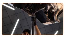
Install the exhaust system fastener.
