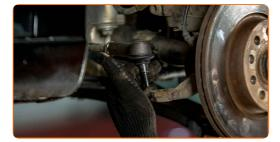
Tighten the fastening nut connecting the tie rod end to the steering knuckle. Use a drive socket #19. Use a torque wrench. Tighten it to 20 Nm torque.+90°
