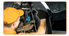
54.1 Install the brake caliper and fix it.
