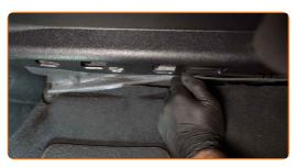
Screw in the fasteners of the bottom trim panel.
