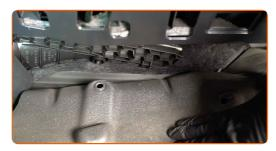
A Remove the cabin filter housing cover.
