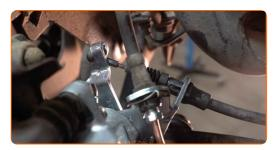
Detach the brake caliper bleed screw cap. Use a crowbar.
