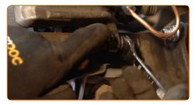
17 Remove the brake caliper.
