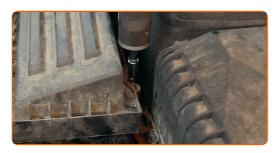
Remove the fender protection cover.
