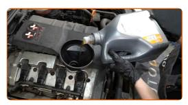
Replacement: engine oil and filter – AUDI TT Coupe (FV3, FVP). AUTODOC recommends:
