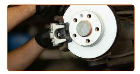
Tighten the brake caliper bracket. Use a combination spanner #15. Use a drive socket #13. Use a torque wrench. Tighten it to 35 Nm torque.
