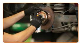
24 Install the brake disc.
