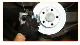
28 Install the brake caliper and fix it.
