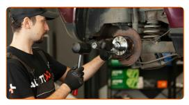
Screw the wheel hub lock nut.
