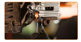
Remove the brake caliper.
