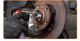
Remove the hub and the bearing together, since they are a sealed unit. Use 3-Arm Gear Puller.
