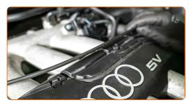
Remove the spark plug wire connectors from the spark plug wells.
