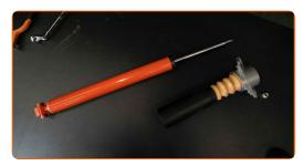
Install the top mount on the new shock absorber and secure it. Use a combination spanner #16. Use an adjustable wrench. Use a torque wrench. Tighten it to 25 Nm torque.
