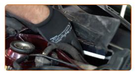
Remove the cabin air filter housing.
