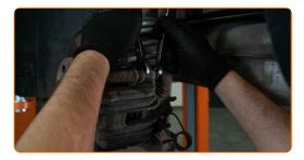
11 Remove the brake caliper.
