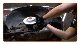
20 Install the brake caliper and fix it.
