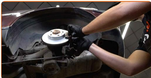
**20** Install the brake caliper and fix it.
