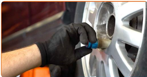
**27** Lower the car and working in a cross order, tighten the wheel bolts. Use a torque wrench. Tighten it to 120 Nm torque.
