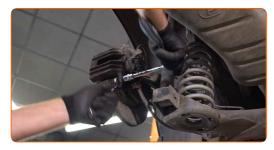
Remove the brake caliper.
