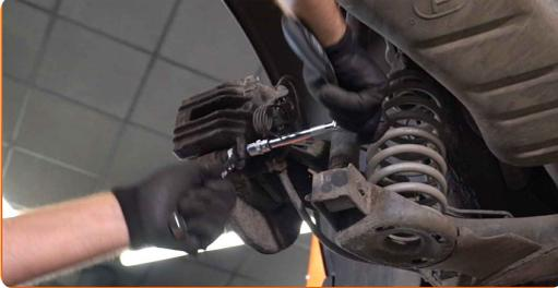
**11** Remove the brake caliper.
