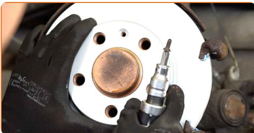
**18** Tighten the brake disc fastening. Use Torx T30. Use a torque wrench. Tighten it to 4 Nm torque.
