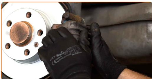
**21** Tighten the brake caliper fasteners. Use a combination spanner #15. Use a drive socket #13. Use a torque wrench. Tighten it to 35 Nm torque.
