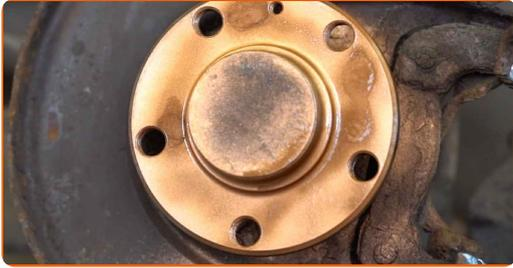
**16** Remove anti-corrosion grease from the new brake disk. Use a brake cleaner.
