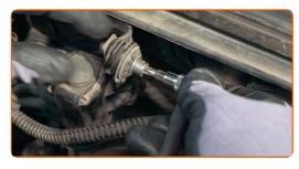
6 Unscrew the brake fluid reservoir cap.
