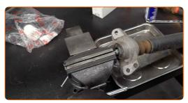
Remove the shock absorber piston rod fastening. Use a combination spanner #14.
