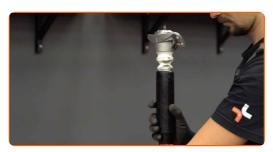
Fix the shock absorber mount. Use a combination spanner #14. Use a drive socket #14. Use a torque wrench. Tighten it to 25 Nm torque.
