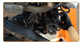
Unscrew the lower fastener of the shock absorber. Use a drive socket #21. Use a tap wrench.
