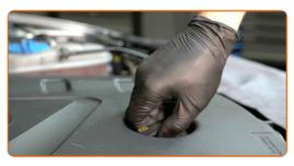
Tighten the oil filler cap.
