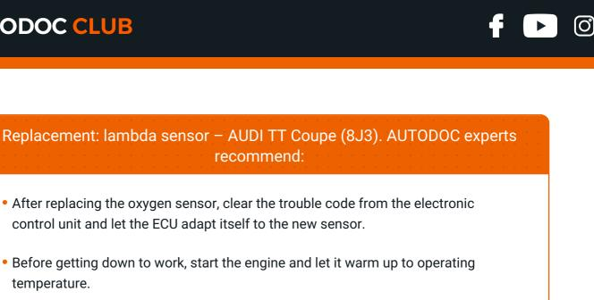
• Please note: all work on the car – AUDI TT Coupe (8J3) – should be done with the engine switched off.
