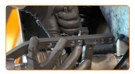
Remove the CV joint together with its boot.
